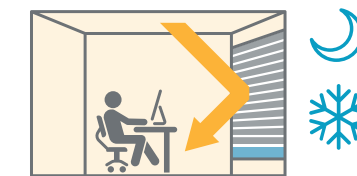
Lowered coverings help prevent heat loss on cooler days during nighttime hours.
