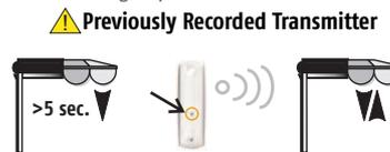
The end product moves for 5 seconds in one direction, to indicate that the dual power cut has been recorded. The motor is in **PROGRAMMING MODE** for 2 minutes.
