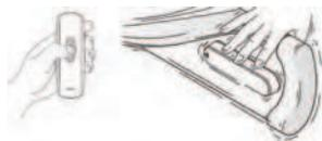
**STEP 7 :** Bring the awning back out and test it again. You can use the remote to stop the awning after 5 seconds (second test mode).
