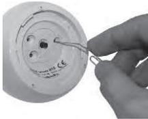
**STEP 3:** Press the PROGRAMMING BUTTON on the back of the Sunis until the awning jogs.
