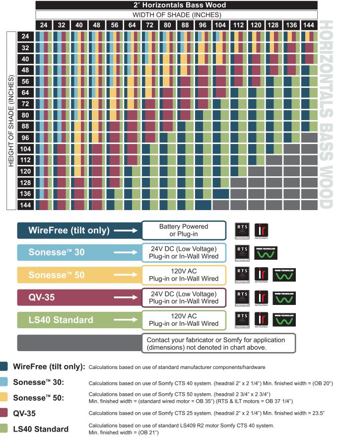
Above chart calculations are based on use of 2 inch Bass Wood horizontal blind slats (approx. .455 lbs./sq ft.) and associated bottom bar/weights.
