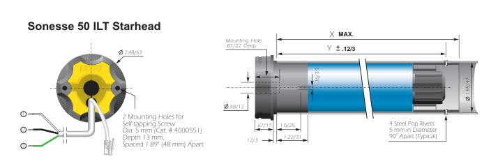
NOTE: Both cables can be removed from motor for servicing.
