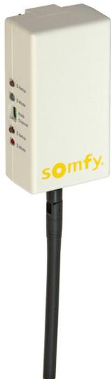
The Z-Wave® to Radio Technology Somfy® Interface (ZRTSI) is a Z-Wave bridge controller that receives Z-Wave transmissions and converts them to motor commands for Somfy's full range of interior and exterior RTS wireless controlled motors.
